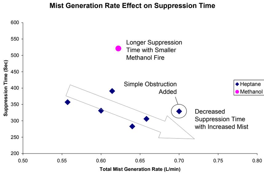
**Figure 4. The extinguishment times as a function of total mist generation rate**
