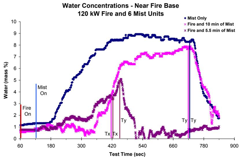
**Figure 6. Water mass concentration from several 6 mist unit tests**
