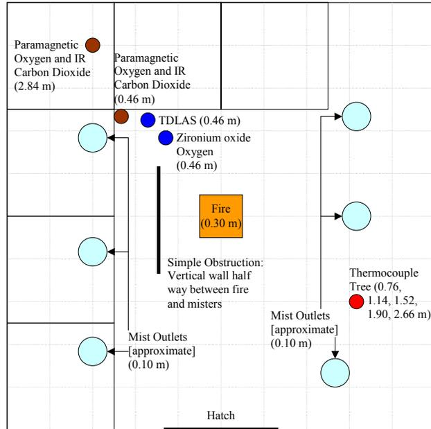
**Figure 3. 28 m<sup>3</sup> compartment layout**
