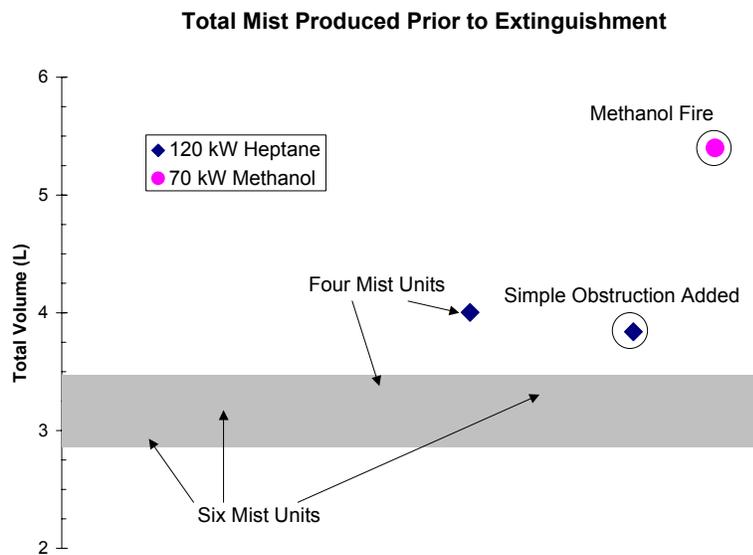
**Figure 5. The total volume of mist produced prior to extinguishment for the tests**
